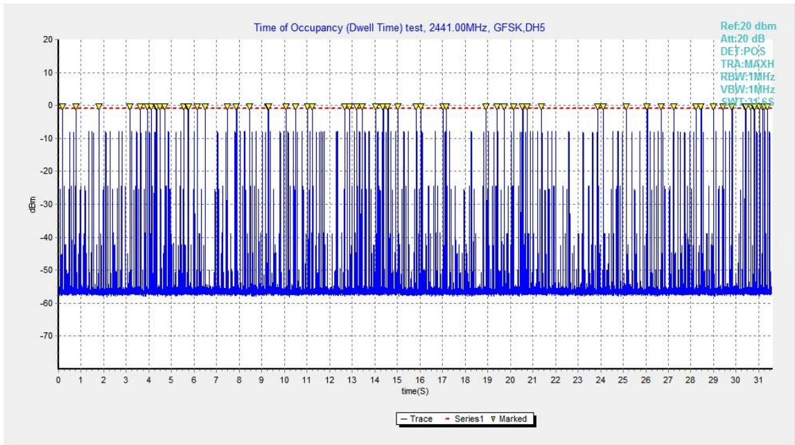
Fig.69. Number of Transmissions Measurement: Channel 39,Packet DH5
