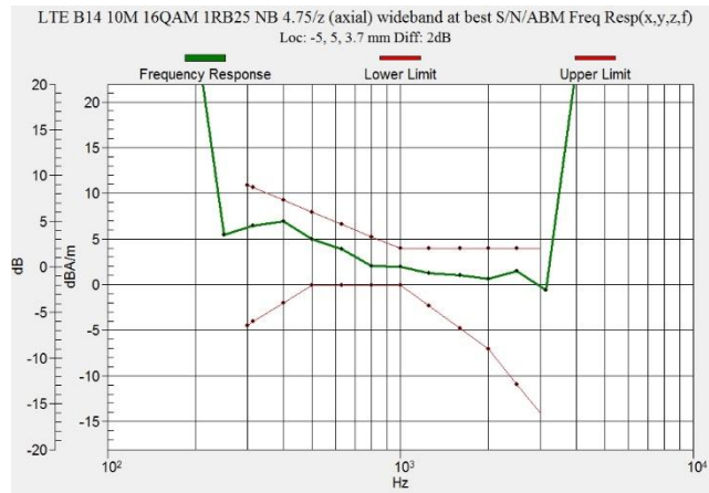
Figure C.10 Frequency Response of LTE B14
