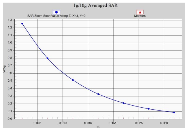
Fig.A.1- 18 Z-Scan at power reference point (LTE band4) 15mm
