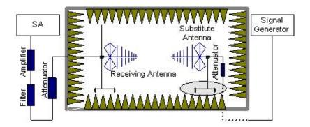
In the chamber, an substitution antenna for the frequency band of interest is placed at the reference point of the chamber. An RF Signal source for the frequency band of interest is connected to the substitution antenna with a cable that has been constructed to not interfere with the radiation pattern of the antenna. A power ( $P_{\text{Mea}}$ ) is applied to the input of the
