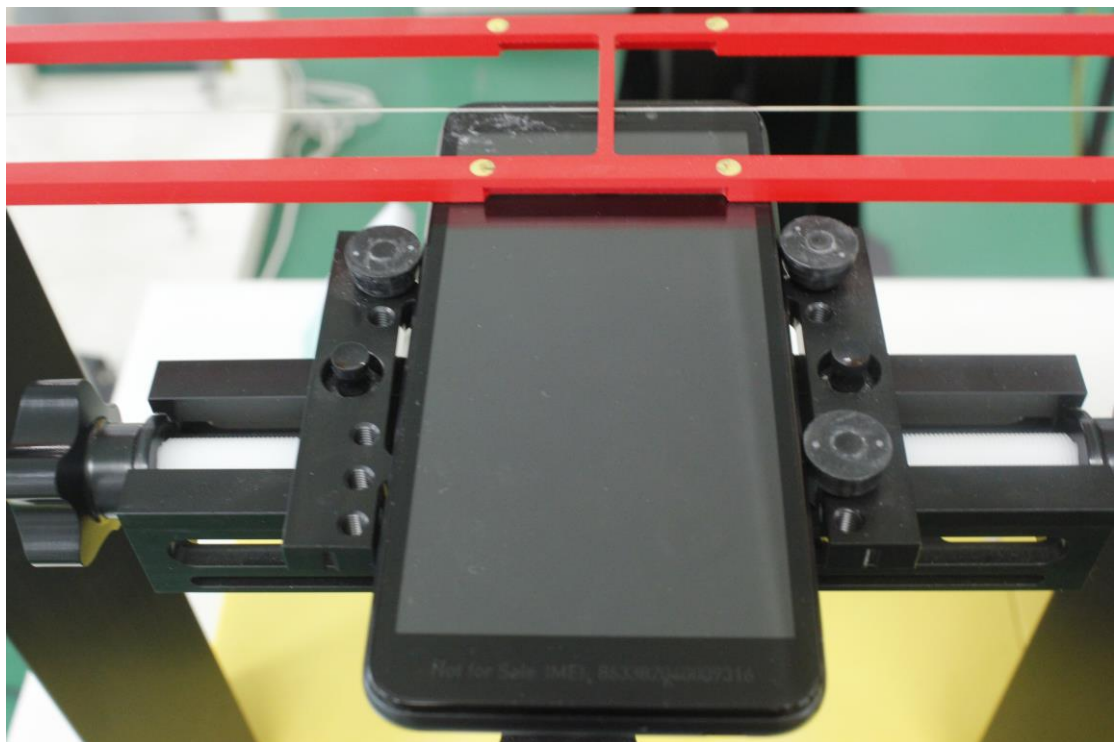
Picture 2: EUT Positioning for RF/T-coil
