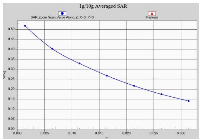
Fig.A.1- 23 Z-Scan at power reference point (LTE band12)
