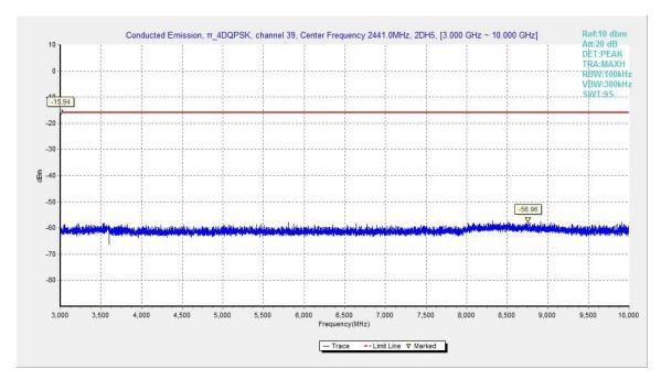
Fig.36. Conducted spurious emission: π/4 DQPSK, Channel 39, 3GHz - 10GHz
