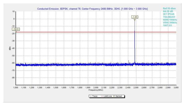
Fig.55. Conducted spurious emission: 8DPSK, Channel 78, 1GHz - 3GHz
