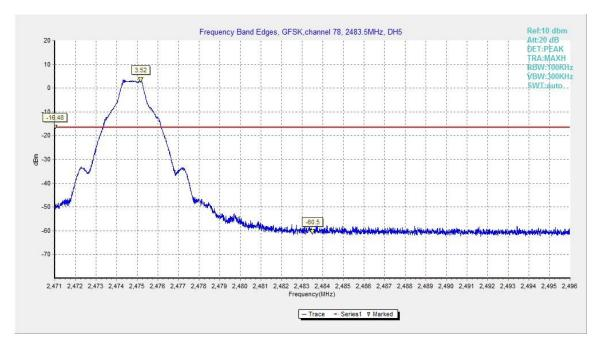
Fig.3. Frequency Band Edges: GFSK, Channel 78, Hopping Off
