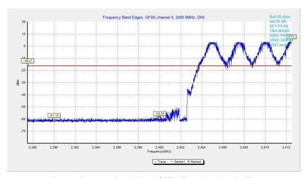
Fig.2. Frequency Band Edges: GFSK, Channel 0, Hopping On
