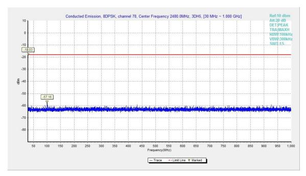
Fig.54. Conducted spurious emission: 8DPSK, Channel 78, 30MHz - 1GHz
