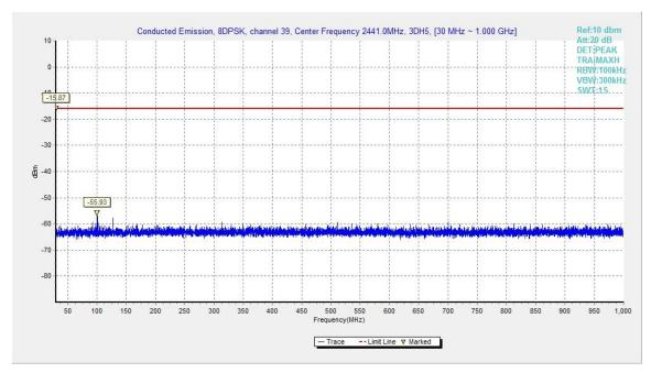
Fig.49. Conducted spurious emission: 8DPSK, Channel 39, 30MHz - 1GHz
