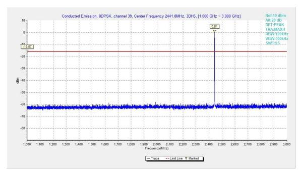
Fig.50. Conducted spurious emission: 8DPSK, Channel 39, 1GHz - 3GHz
