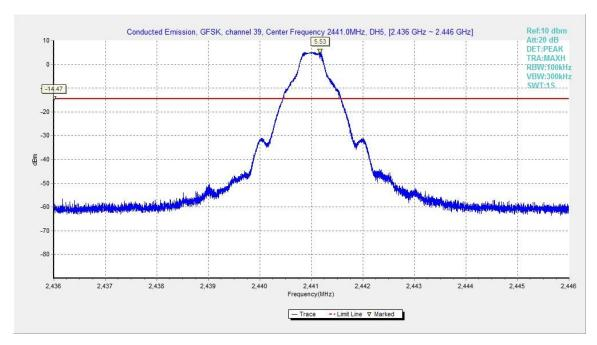
Fig.18. Conducted spurious emission: GFSK, Channel 39, 2441MHz
