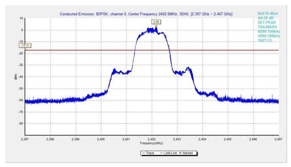
Fig.43. Conducted spurious emission: 8DPSK, Channel 0,2402MHz
