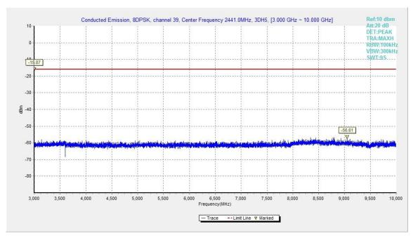
Fig.51. Conducted spurious emission: 8DPSK, Channel 39, 3GHz - 10GHz
