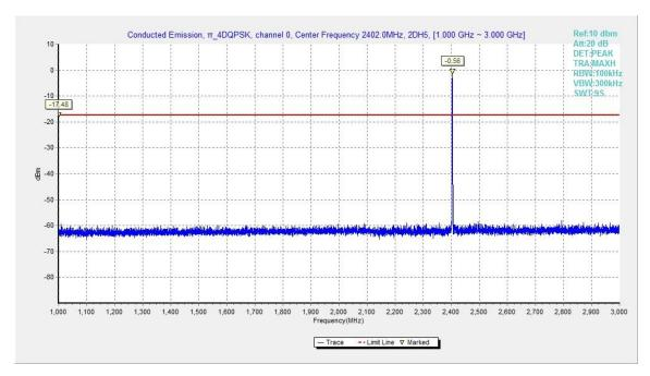
Fig.30. Conducted spurious emission: π/4 DQPSK, Channel 0, 1GHz - 3GHz
