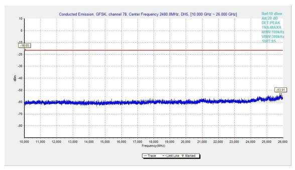
Fig.27. Conducted spurious emission: GFSK, Channel 78, 10GHz - 26GHz
