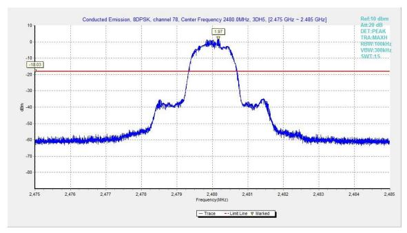
Fig.53. Conducted spurious emission: 8DPSK, Channel 78, 2480MHz
