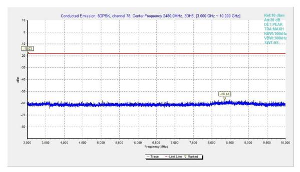
Fig.56. Conducted spurious emission: 8DPSK, Channel 78, 3GHz - 10GHz
