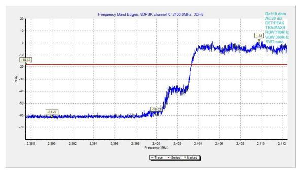
Fig.10. Frequency Band Edges: 8DPSK, Channel 0, Hopping On
