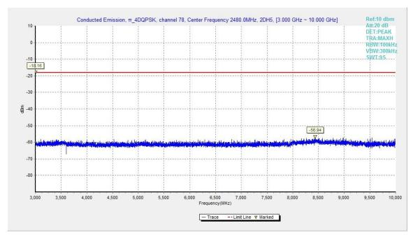
Fig.41. Conducted spurious emission: π/4 DQPSK, Channel 78, 3GHz - 10GHz
