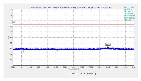
Fig.26. Conducted spurious emission: GFSK, Channel 78, 3GHz - 10GHz
