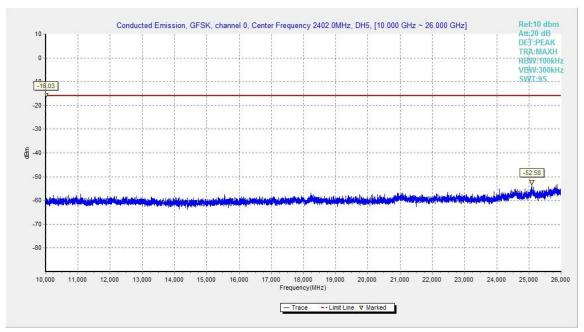
Fig.17. Conducted spurious emission: GFSK, Channel 0,10GHz - 26GHz
