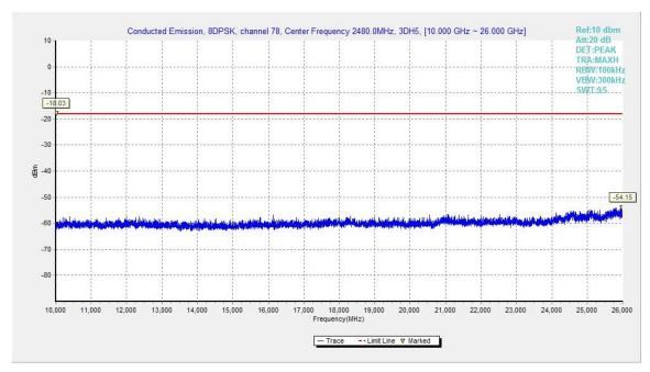
Fig.57. Conducted spurious emission: 8DPSK, Channel 78, 10GHz - 26GHz
