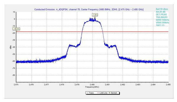
Fig.38. Conducted spurious emission:  $\pi/4$  DQPSK, Channel 78, 2480MHz
