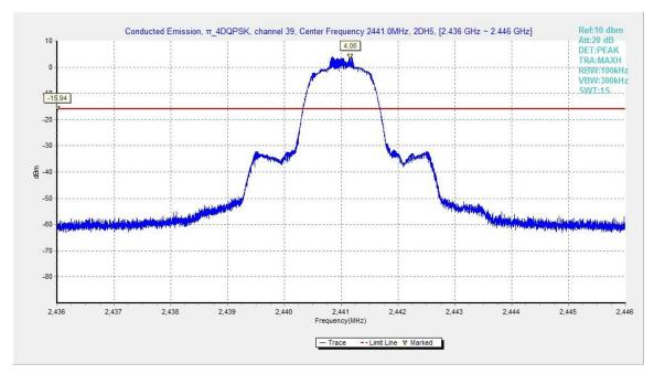
Fig.33. Conducted spurious emission: π/4 DQPSK, Channel 39, 2441MHz
