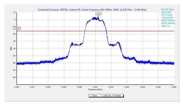
Fig.48. Conducted spurious emission: 8DPSK, Channel 39, 2441MHz
