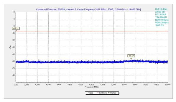
Fig.46. Conducted spurious emission: 8DPSK, Channel 0, 3GHz - 10GHz
