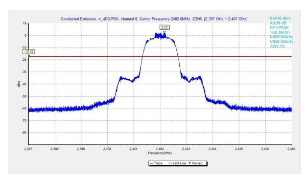
Fig.28. Conducted spurious emission:  $\pi/4$  DQPSK, Channel 0,2402MHz
