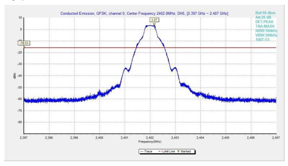
Fig.13. Conducted spurious emission: GFSK, Channel 0,2402MHz
