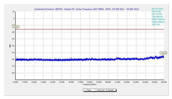
Fig.52. Conducted spurious emission: 8DPSK, Channel 39, 10GHz – 26GHz
