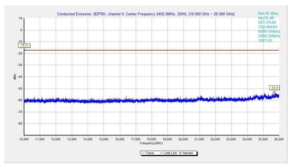
Fig.47. Conducted spurious emission: 8DPSK, Channel 0,10GHz - 26GHz
