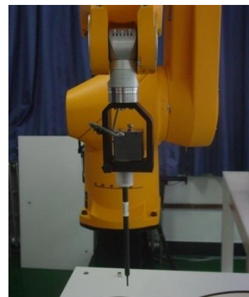
Picture C.2 Near-field Probe
