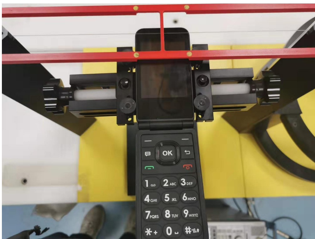
Picture 2: EUT Positioning for RF/T-coil
