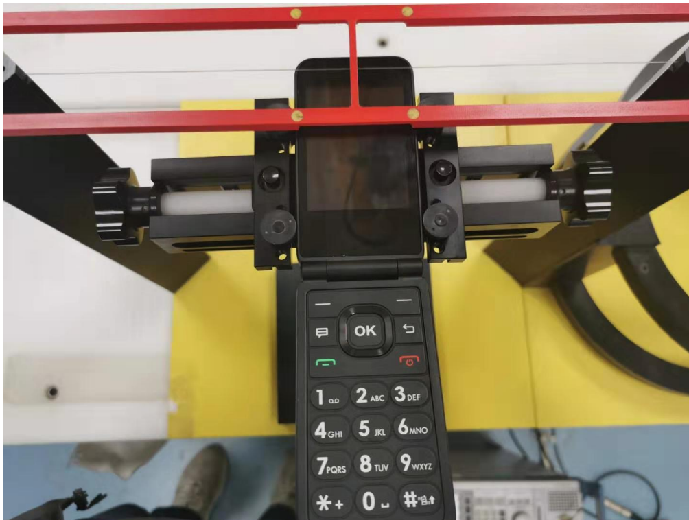
Picture 2: EUT Positioning for RF/T-coil
