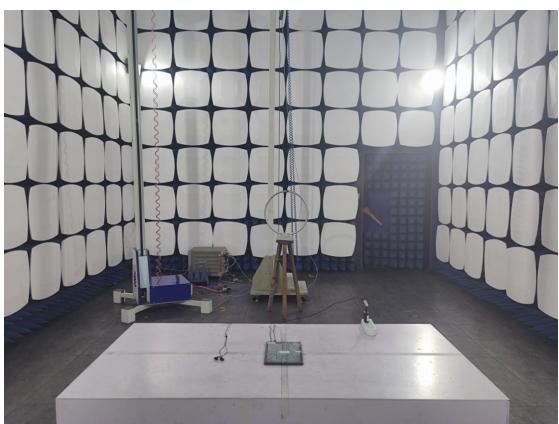
3. Radiated emission (9KHz-30MHz)
