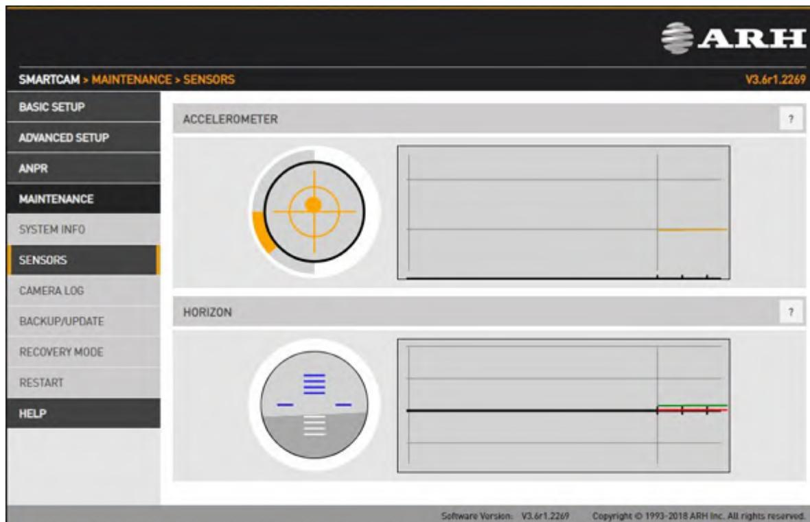
The built-in accelerometer may provide help aligning the camera.
