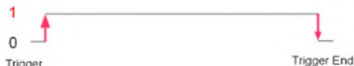
**Start/end offset:** the interval during which the trigger is asserted can be extended in both directions with start and end offsets.
