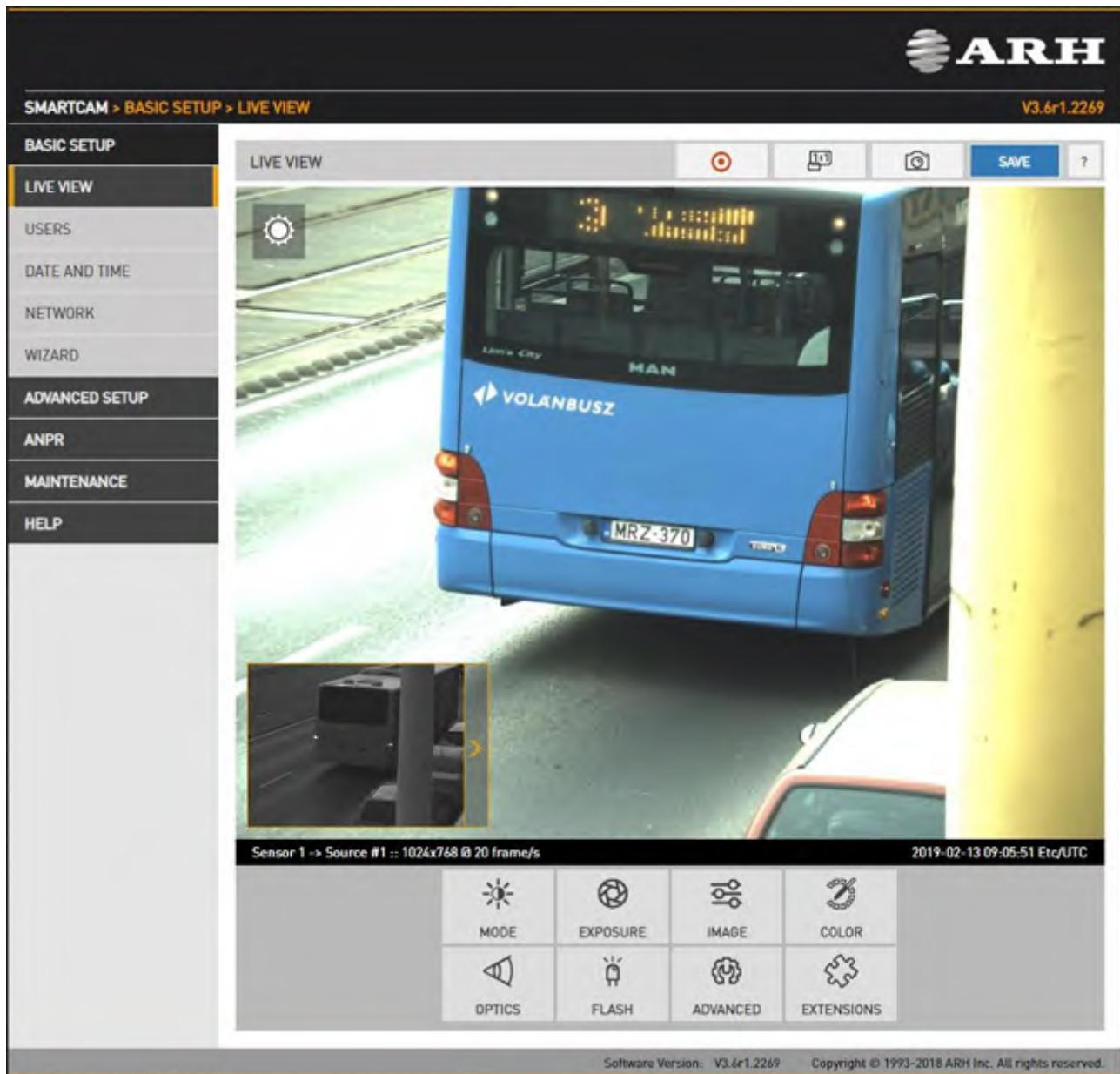
The live stream of the secondary sensor is shown in the box below (picture in picture). By clicking the live stream box, the main view switches to the secondary sensor, and all settings (Brightness control, Color, etc.) will be applied to the secondary sensor.
