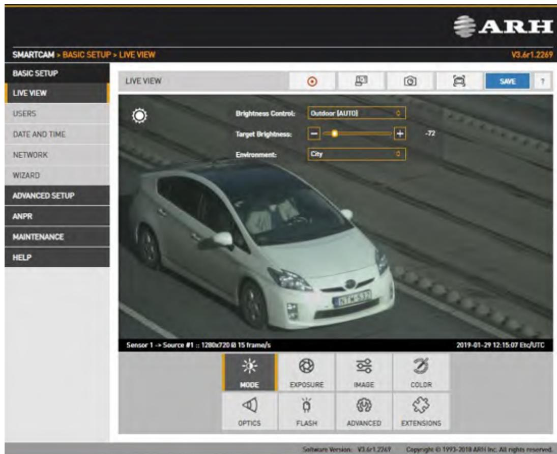
Brightness control will automatically monitor and control the exposure of the image, with license plate reading as a priority.
