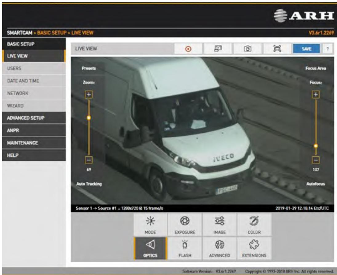
Models equipped with motorized lenses will show this menu item. Use the left slider (Zoom) to change the field of view from wide angle (0) to telephoto (100). Use the right slider (Focus) to manually adjust focus from near to far.
