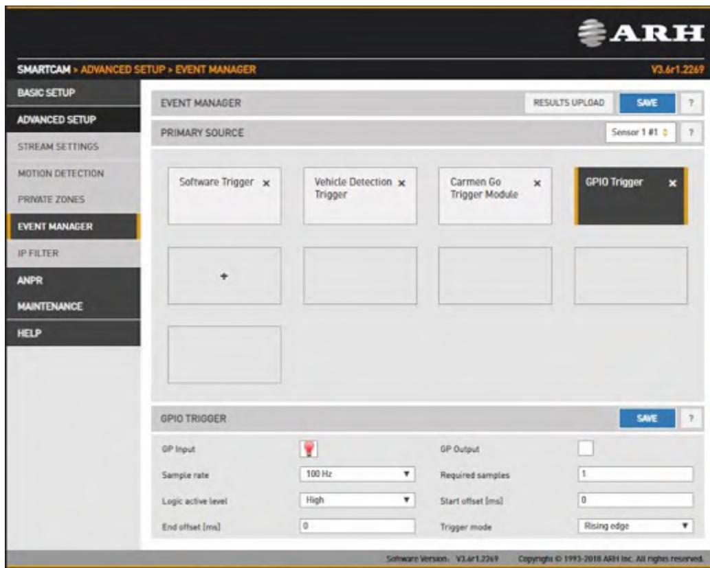
GPIO Trigger is a hardware trigger source accepting triggers from one of the General Purpose (GP) Inputs of the device. Please refer to the Install Guide for details of the electric connection.
