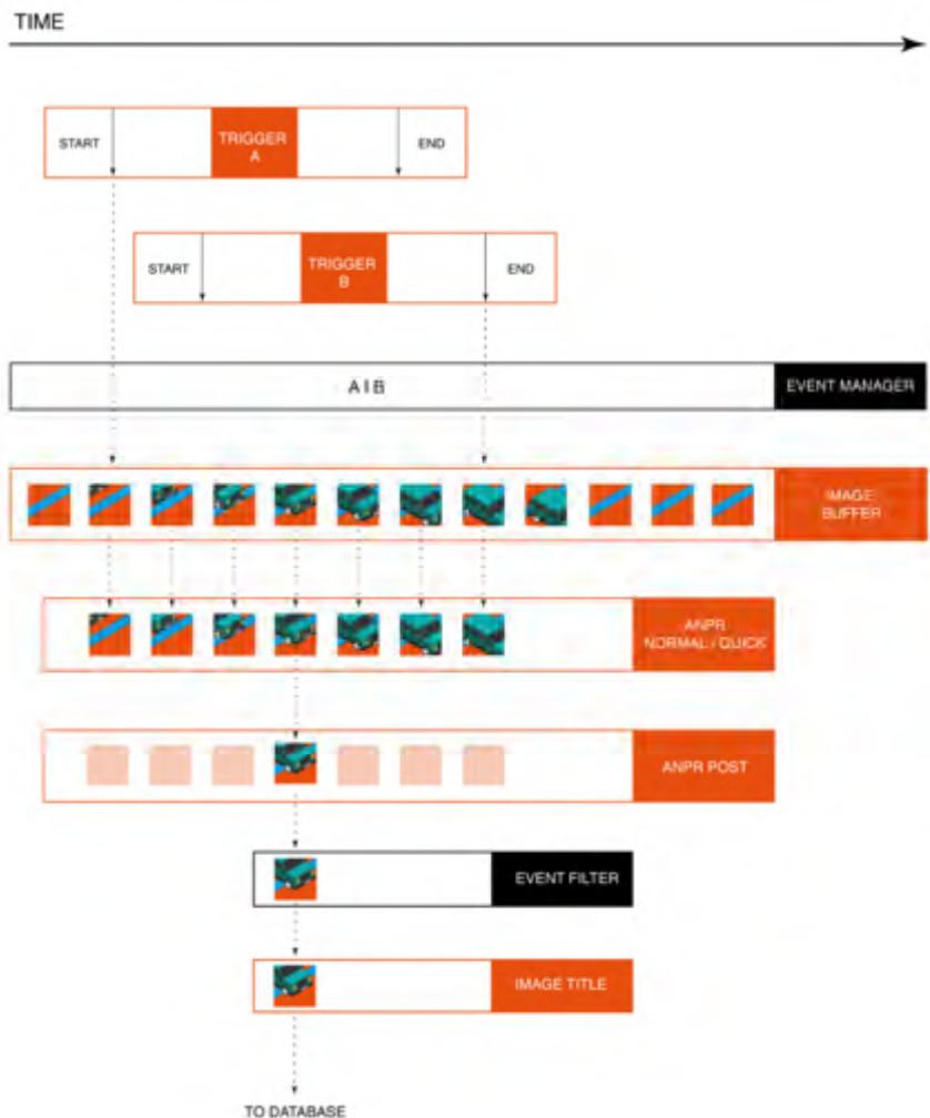
The above graphic is the schematic overview of trigger events being processed. License plate recognition operates as a multistage pipeline, taking a sequence of images of the same event as input, producing one image of the vehicle (with the license plate in the best position), license plate and event data (textual form), and a license plate image as an output.
