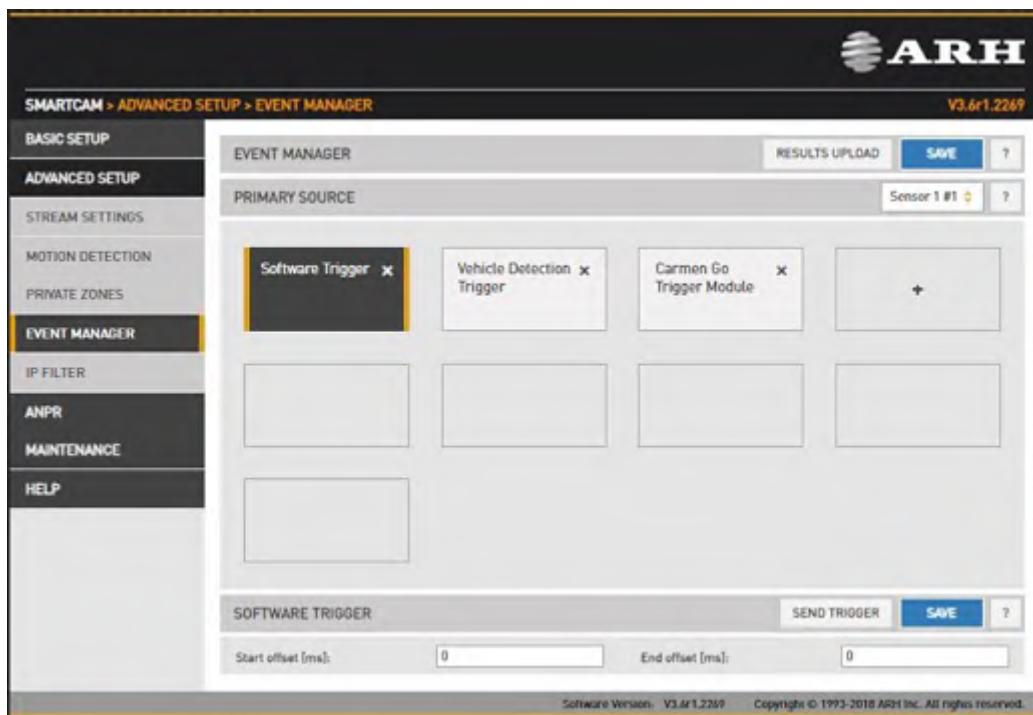
A software trigger is an external trigger sent as a HTTP request.
