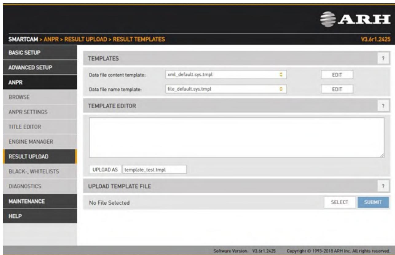
The content of the result data file (and the file name) is customizable using templates. The following short example, which will describe a result formatted as an XML contains all features:
