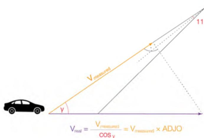
However, the actual speed can be calculated if the pan and tilt angles of the device are known (see images above). The measured speed can be corrected if the two parameters above (ADJO and ADJL) are determined on the basis of the angles.
