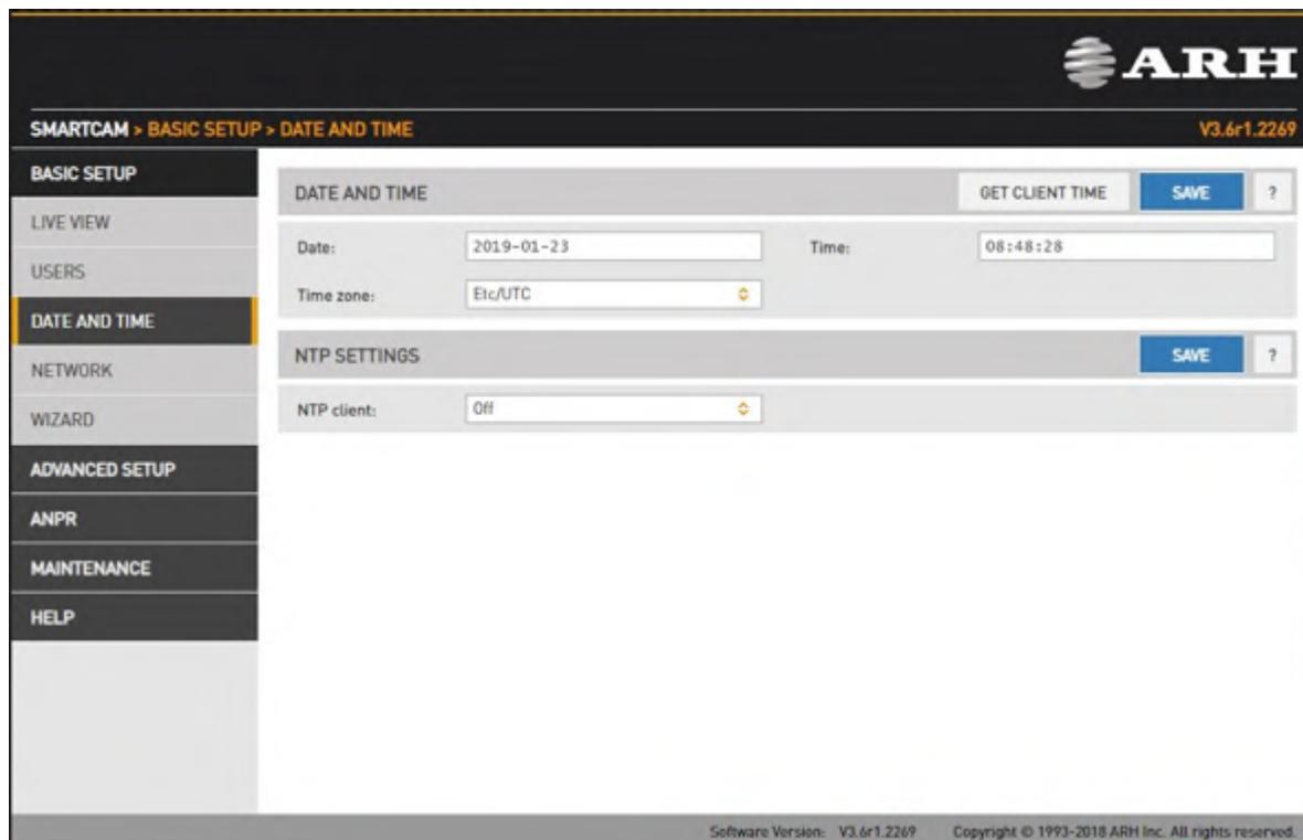
Current date and time and timekeeping settings are managed in this page. Users can choose to set date and time manually once or to use a time synchronization protocol (NTP), which will keep time synchronized to a server over network.
