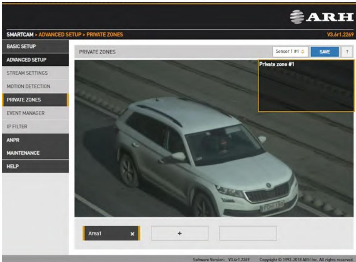
In certain circumstances it may be necessary to cover a part of the image, for instance, a parking place near the monitored lane, where the stationary vehicles should not be in the image, and their license plates should be excluded from processing, or when private property is displayed. These unwanted parts can be covered with max. 3 rectangular patches with the Private zones tool.
