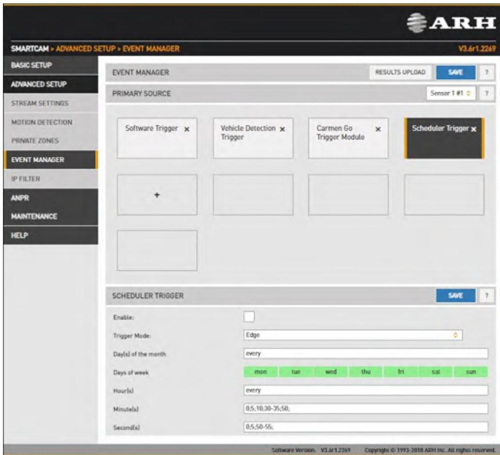
This trigger source provides the user with a timer. Triggers can be scheduled with a precision of one second. Two trigger modes are available:
