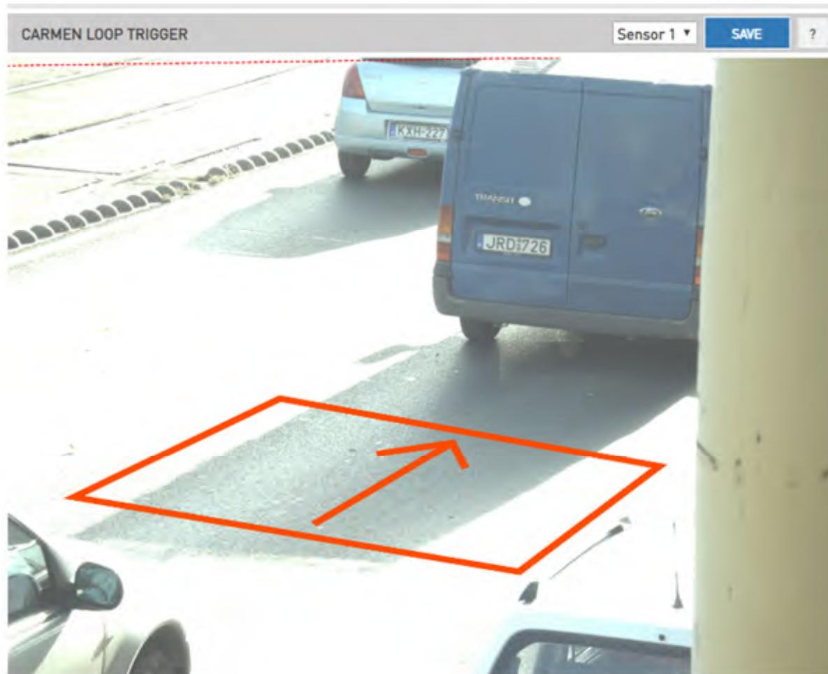
The arrow in the rectangle must show the direction of the passing cars. **If the arrow is not moving towards the direction of the cars, use the left mouse button to click the rectangle to rotate the arrow.**
