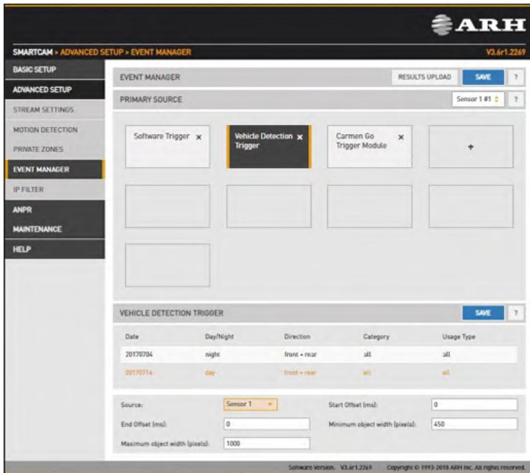
The Vehicle Detector is an image processing algorithm capable of detecting and tracking a vehicle in a stream of images. You can monitor detected vehicles at the Live View menu by clicking the
