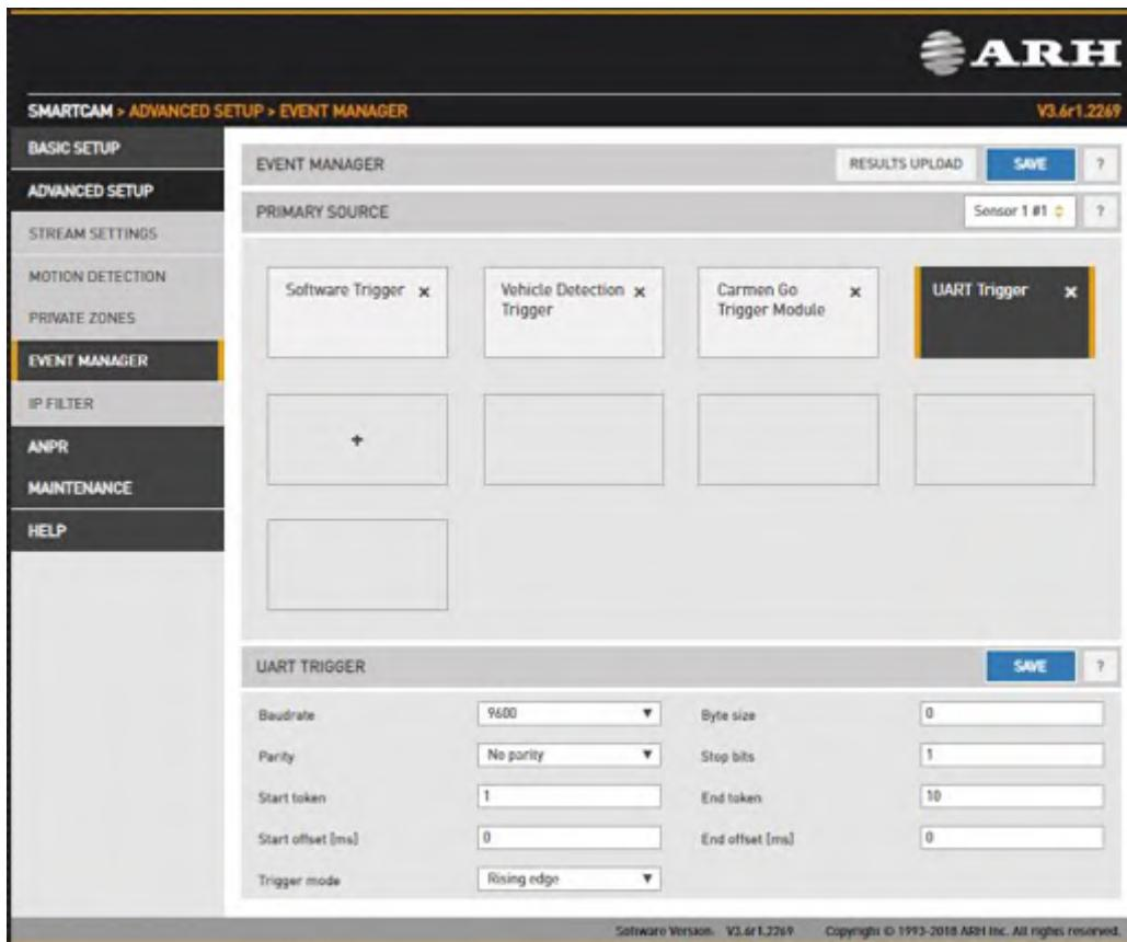
The camera can be triggered through its UART port. Besides the common UART properties (**Baudrate**, **Byte size**, number of **Parity** bits, and **Stop bits**) the communication protocol can also be specified here. A UART trigger event starts with a Trigger **Start Token** (TST) byte, then max. 254 bytes of trigger data may follow, and then it ends with a Trigger **End Token** (TET) byte.
