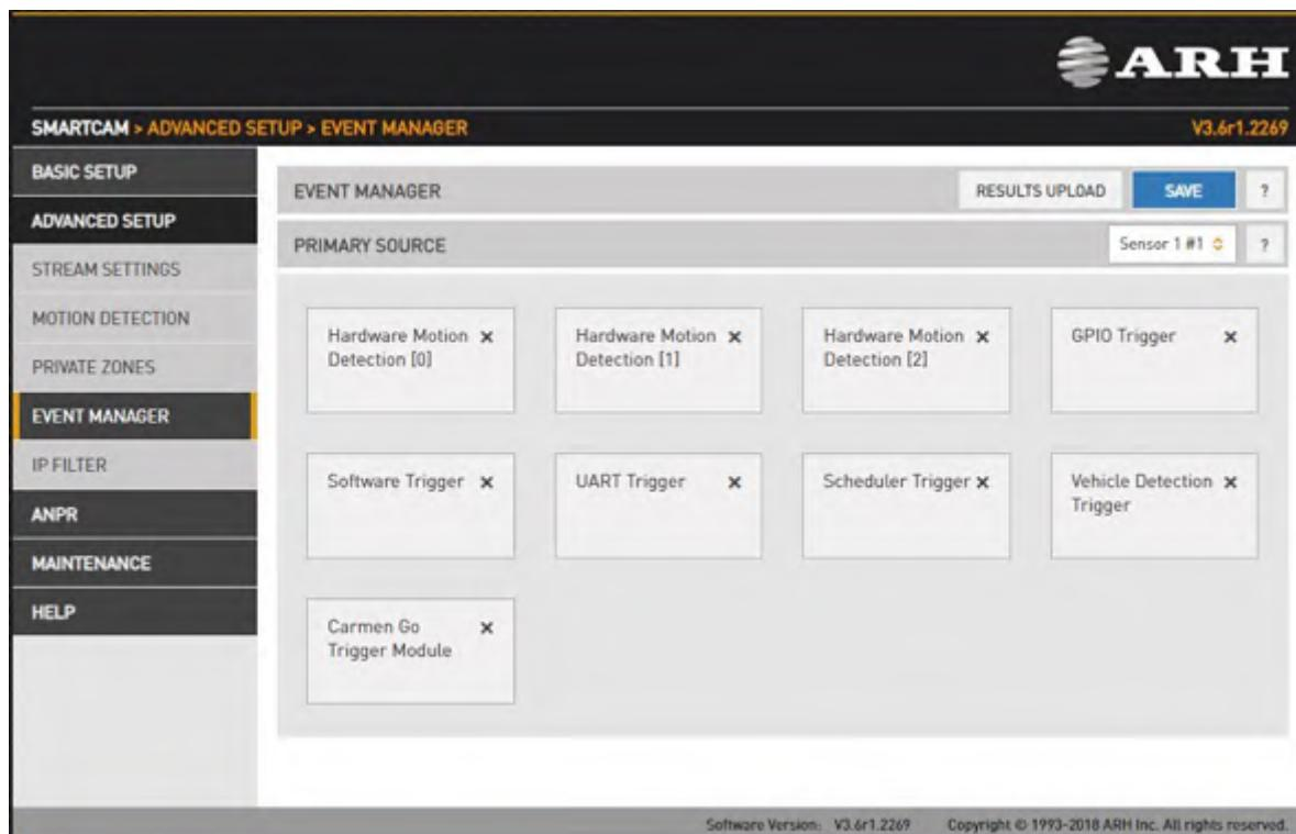
You can add and remove trigger sources in this menu. Clicking the + icon, you will be presented all available trigger sources. The sources will be connected with an OR conjunction: the trigger will be asserted while any of the trigger sources are active. Selecting a trigger source its configuration will be available at the bottom of the screen.
