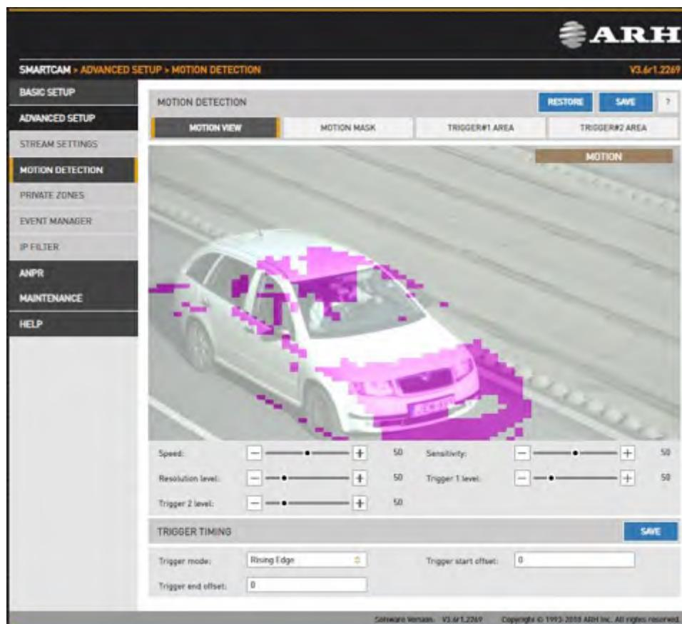
The motion detector can provide three trigger sources:
