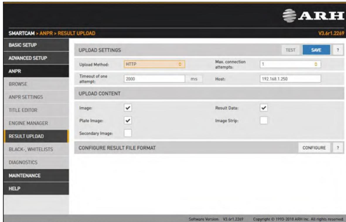
Recognition results can be uploaded using the HTTP, FTP or SFTP protocol.
