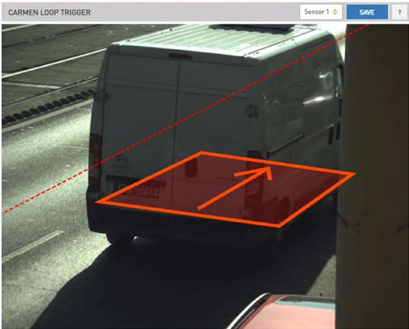
You can rotate the lane line **by right-clicking the button and pressing the left mouse button**. At this time, the lane line starts to rotate. If the lane line is roughly parallel to the band, release the left mouse button. Right-click to move more positioning.
