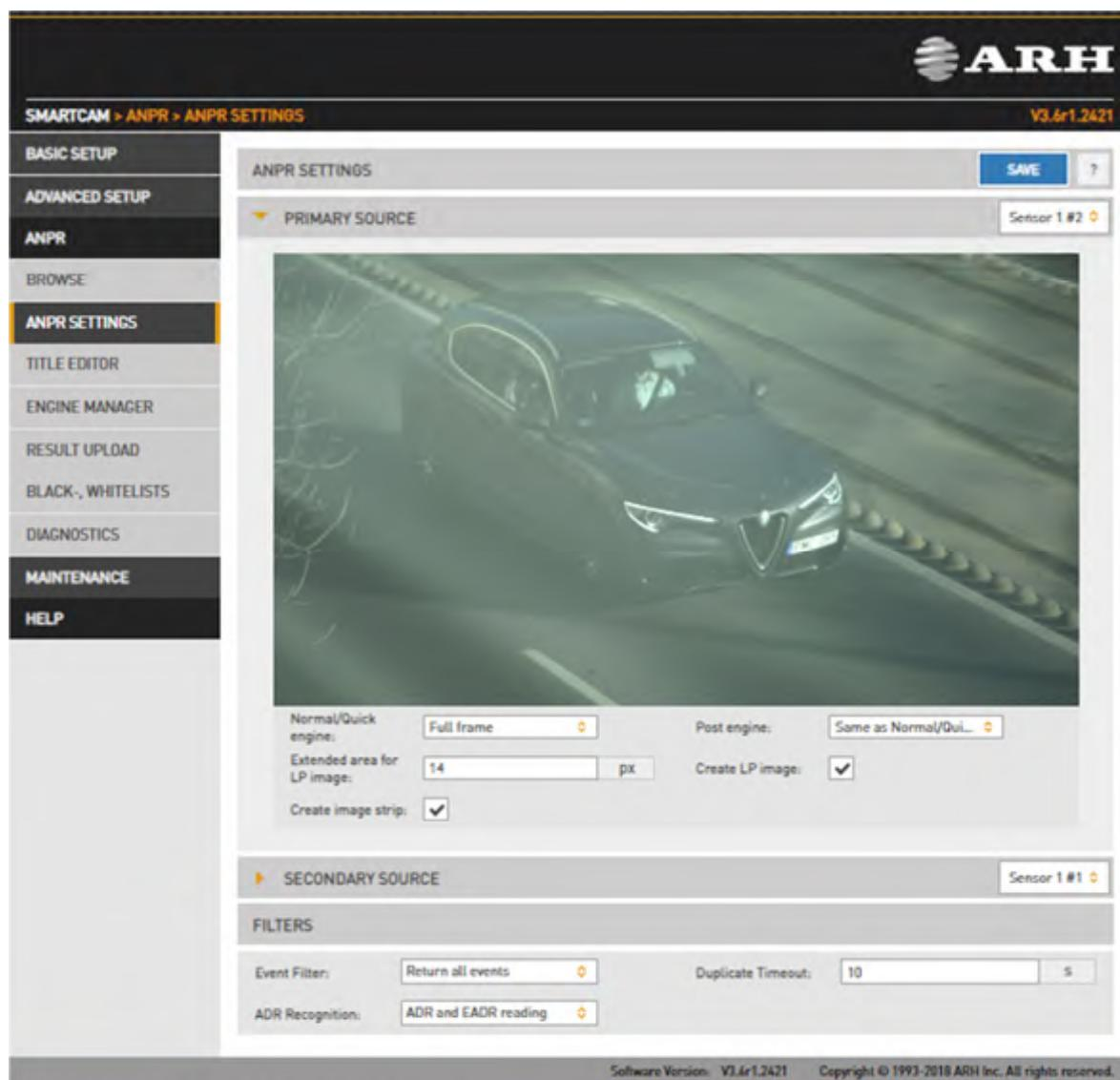
The main properties of the license plate recognition pipeline are configured here.
