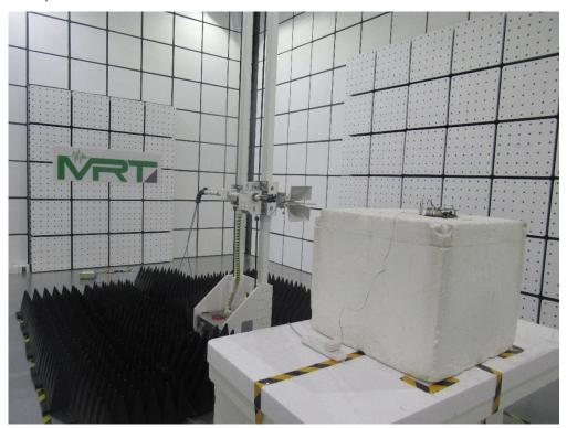
Description: Radiated Spurious Emission Test Setup for  $1GHz \sim 18GHz$  (The testing distance is 3m)
