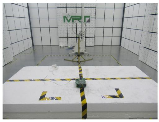
Description: Radiated Spurious Emission Test Setup for  $30 \text{MHz} \sim 1 \text{GHz}$
