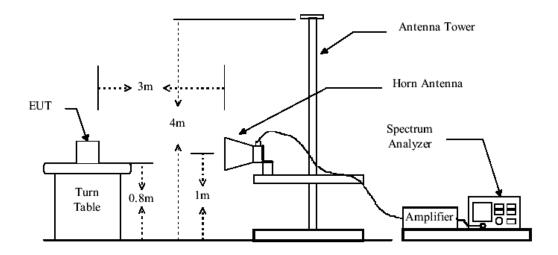
Low nosie amplifier was used below 1GHz, High pass Filter was used above 1GHz.
