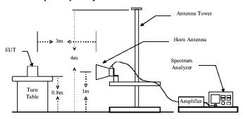
The field strength is calculated by adding the Antenna Factor, Preamplifier Factor & Cable Factor. The basic equation with a sample calculation is as follows:
