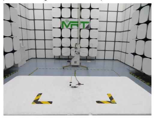
Description: Radiated Emission Test Setup for above 1GHz (HSBT3008-EA Configured External PCB Antenna)
