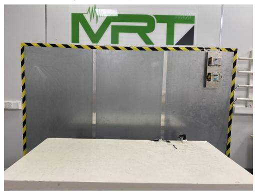
Description: Back View of Conducted Emission Test Setup for Power Port (HSBT3008-EA Configured External Dipole Antenna)
