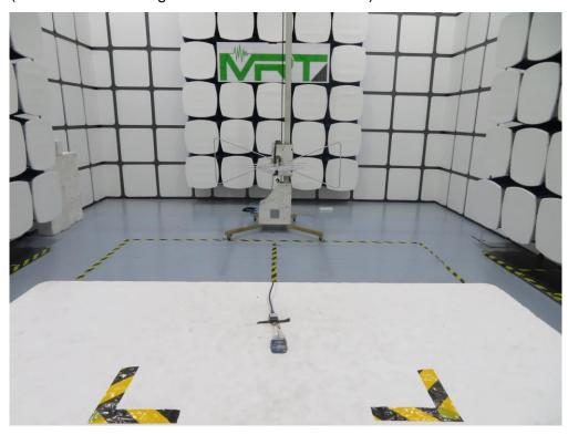
Description: Radiated Emission Test Setup for above 1GHz (HSBT3008-IA Configured Onboard PCB Antenna)
