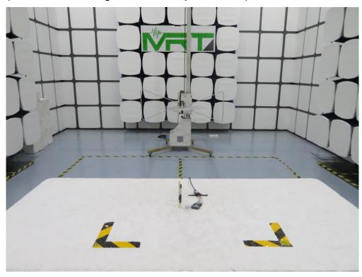
Description: Radiated Emission Test Setup for above 1GHz (HSBT3008-EA Configured External Dipole Antenna)
