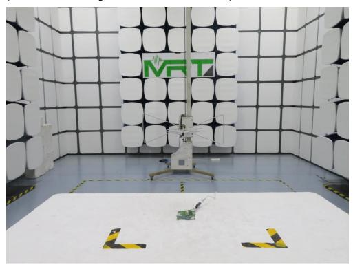
Description: Radiated Emission Test Setup for above 1GHz (HSBT3007-IA Configured Onboard PCB Antenna)
