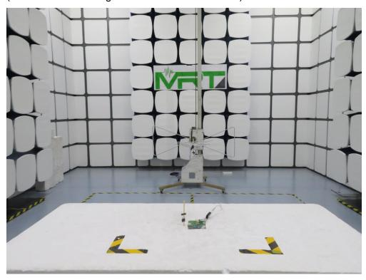
Description: Radiated Emission Test Setup for above 1GHz (HSBT3007-EA Configured External PCB Antenna)
