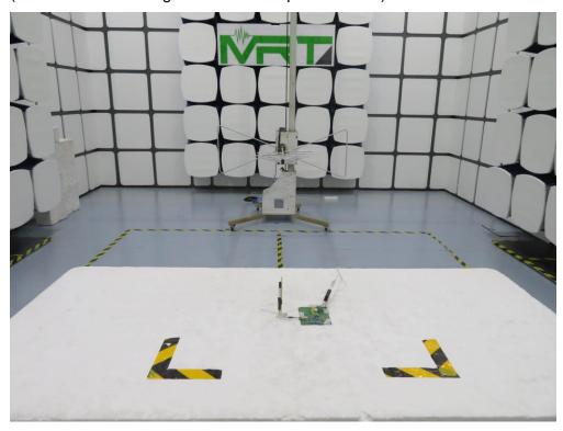
Description: Radiated Emission Test Setup for above 1GHz (HSBT3007-EA Configured External Dipole Antenna)
