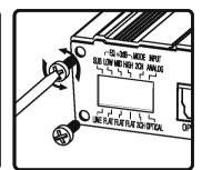
3. To attach mounting bracket, remove all faceplate screws from one side. Lift faceplate and set aside.
