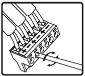
1. to connect wires to the Euro-Block connector loosen the screws, insert a 1/4" in of stripped wire and tighten the screws.
