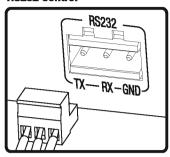
1. Connect the RS232 control device to the RS232 port on the SB335. Refer to Step 1 of "Speaker Connections" for instructions on wiring the Euro-Block connector.
