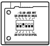
3. To boost the mid frequencies and increase intelligibility set Dip switch 3 to the up position (+3dB)
