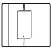
7. The power supply can be attached to a mounting surface using the Velcro strips.
