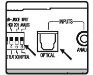
1. For digital connections connect an optical cable from your source to the optical input on the SB335. Set dip switch 6 in the down position.
