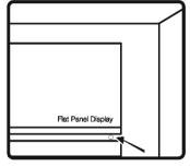
2. Position the IR receiver on a surface that faces out into the area you will be using the remote control. Fasten the IR receiver with the supplied two-sided tape disk.
