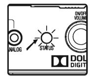
2. Press and hold the mute button on the remote control for 3 seconds then release. The SB335 LED will blink white for 1 minute or until paired.
