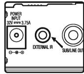
1. Connect the 1/8" mini plug from the IR receiver to the External IR port on the SB335.
