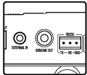
1. Connect a Subwoofer to the SB335 with an Audio BCA cable.
