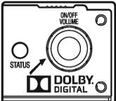
1. Turn the SB335 on by pressing the on/off button. The LED will turn white when on.
