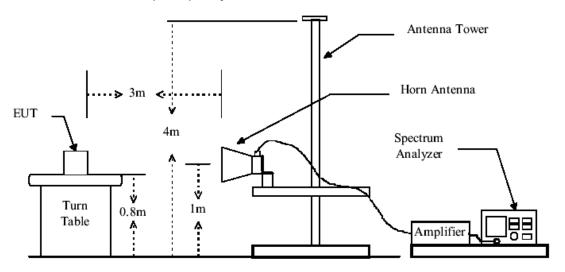
Low nosie amplifier was used below 1GHz, High pass Filter was used above 1GHz.
