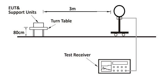
For Radiated emission 30MHz to 1GHz:
