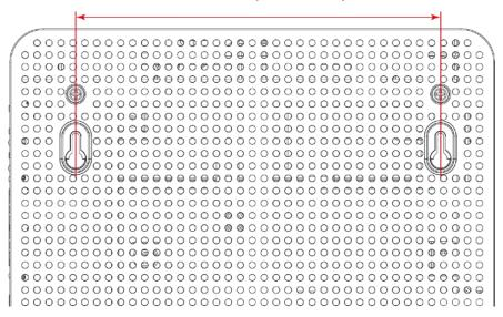
**Note:** The screws should protrude from the wall so you can fit the device between the head of the screws and the wall. If you install the screws in drywall, use hollow wall anchors to ensure the unit does not pull away from the wall due to prolonged strain from the cable and power connectors.
