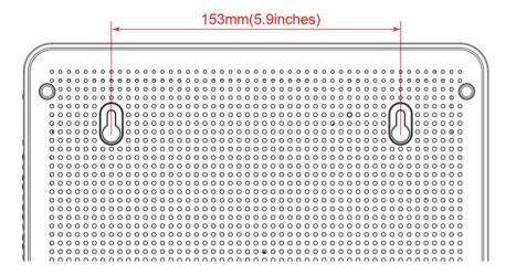
**Note:** The screws should protrude from the wall so you can fit the device between the head of the screws and the wall. If you install the screws in drywall, use hollow wall anchors to ensure the unit does not pull away from the wall due to prolonged strain from the cable and power connectors.
