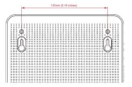
**Note:** The screws should protrude from the wall so you can fit the device between the head of the screws and the wall. If you install the screws in drywall, use hollow wall anchors to ensure the unit does not pull away from the wall due to prolonged strain from the cable and power connectors.
