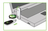
\*Right Angle Connector is needed when inserting the Clear USB into a vertical USB slot.
