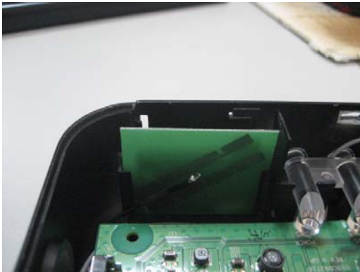
Ant1. Dimension: (L)44mm*(W)35mm*(H)0.8mm Φ1.37mm Cable Length: 142mm (Black)
