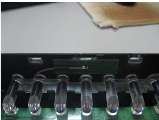
Ant2. Dimension: (L) 41.65*(W)12.25*(H)0.8mm Φ1.37mm Cable Length: 243mm (Gray)
