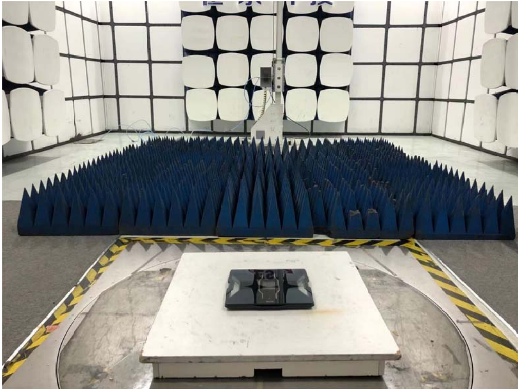
Radiated Test (Above 1GHz)
