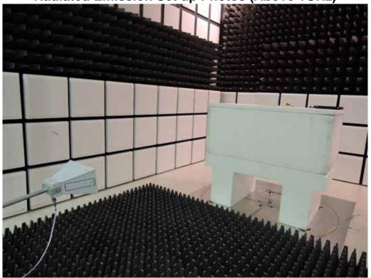
Radiated Emission Set up Photos (Above 1GHz)
