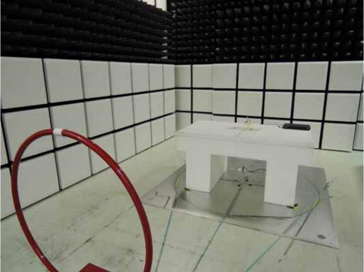
Radiated Emission Set up Photos (Below 1GHz)
