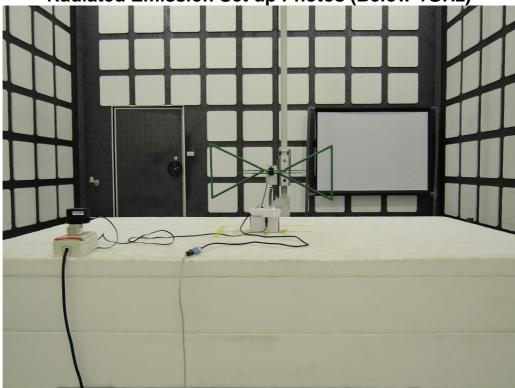
Radiated Emission Set up Photos (Above 1GHz)
