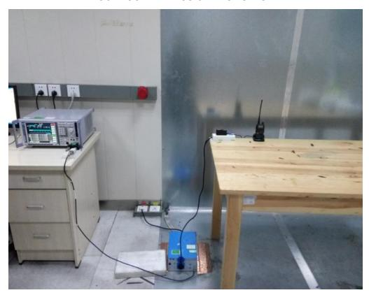
RADIATED EMISSION TEST SETUP
