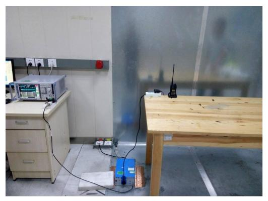
RADIATED EMISSION TEST SETUP
