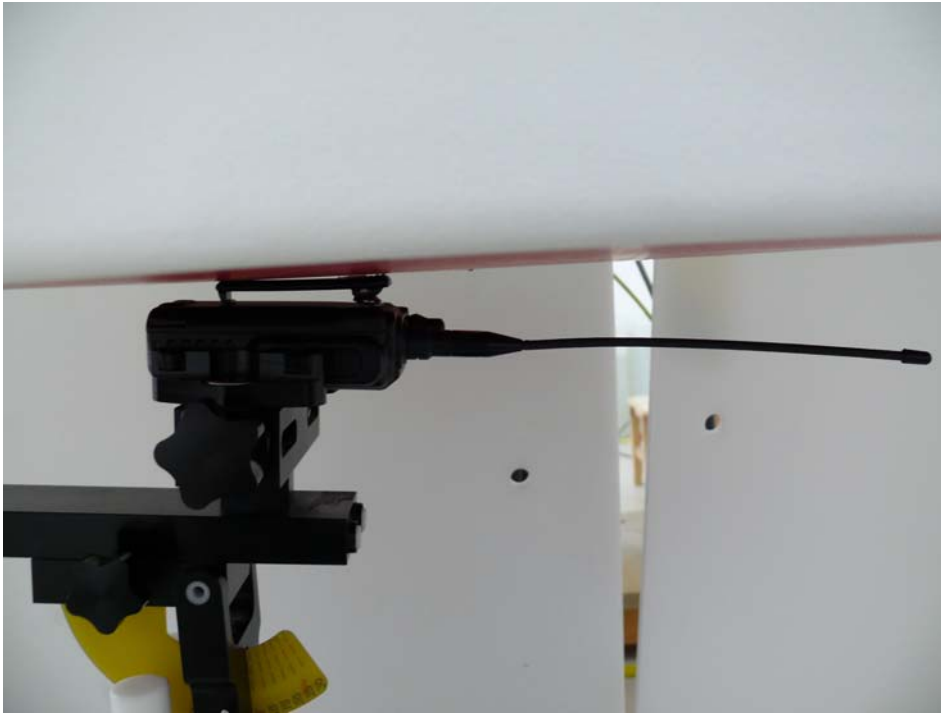
Picture 5: Body-worn, The EUT display towards ground, Belt clip attach the Panantom
