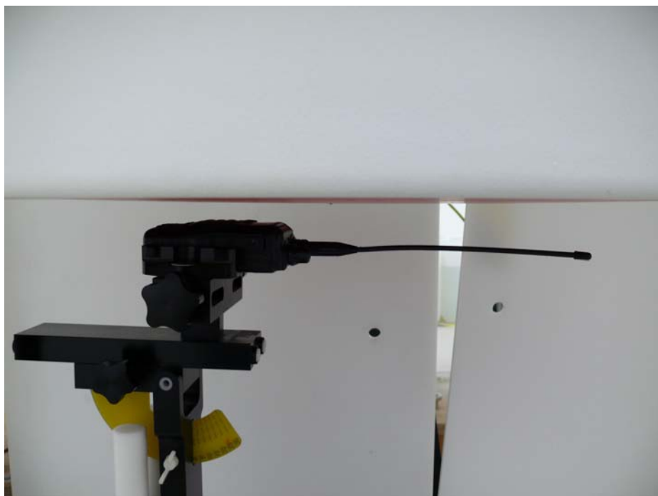
Picture 4: Face-held, The EUT display towards phantom, the distance from EUT to the bottom of the Phantom is 15mm
