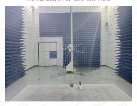
RADIATED EMISSION TEST SETUP-ABOVE 1GHZ
