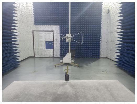
RADIATED EMISSION TEST SETUP ABOVE 1GHz
