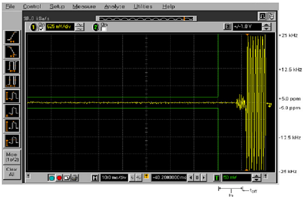
Transmitter Frequency Behavior @ 12.5 KHz Channel Separation--On to Off
