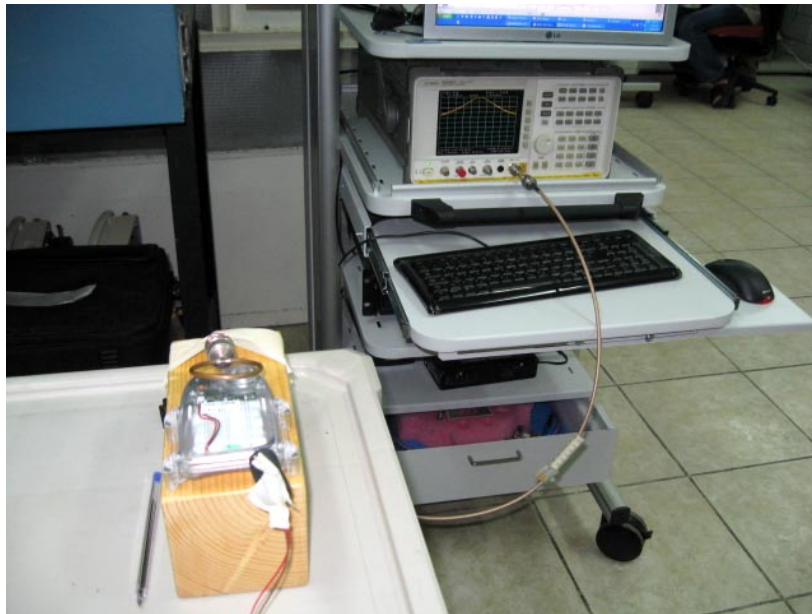
Photograph No.4 Setup for occupied bandwidth measurements
