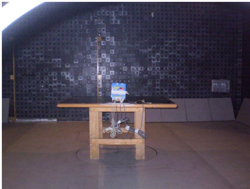
Photograph No.2 Setup for spurious emission measurements in the anechoic chamber below 30 MHz, EUT: sensomatic with internal antenna
