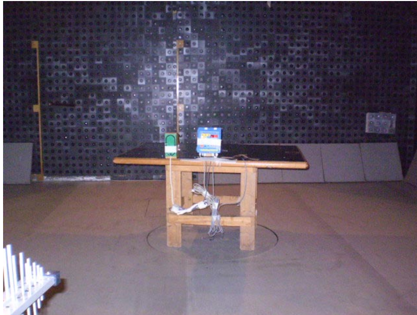
Photograph No.3 Setup for spurious emission measurements in the anechoic chamber from 30 to 1000 MHz, EUT: sensomatic with external antenna
