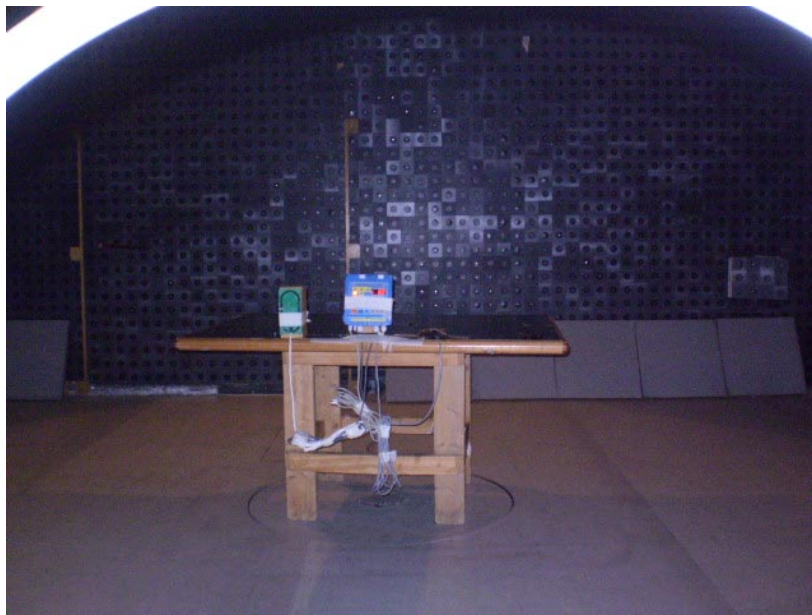
Photograph No.1 Setup for spurious emission measurements in the anechoic chamber below 30 MHz, EUT: sensomatic with external antenna
