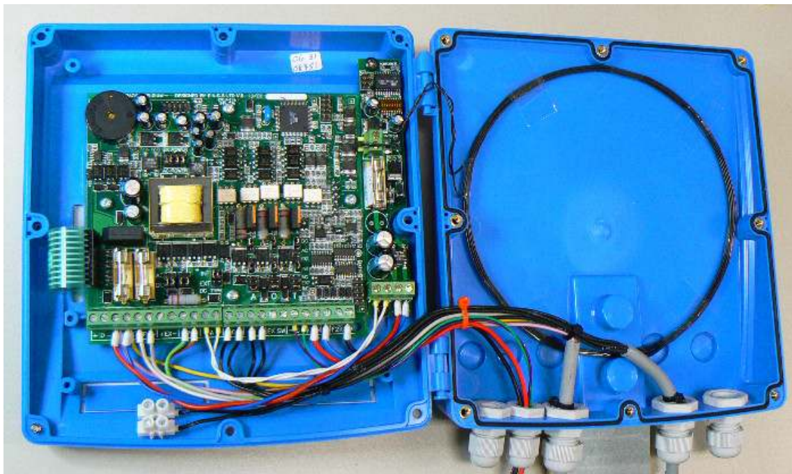
Fig. 3.1 Activator + antenna installed in the Sensomatic enclosure
