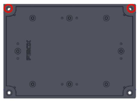
3. Assemble the box brackets, washers, and nuts on the screws and tighten.
