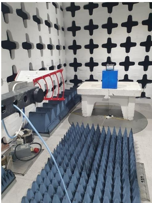
Radiated emissions test set up above 1GHz.
