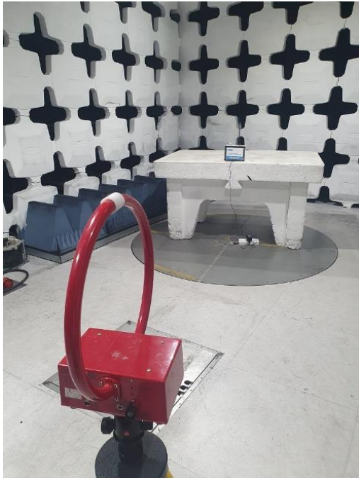
Radiated emissions test set up below 30MHz.
