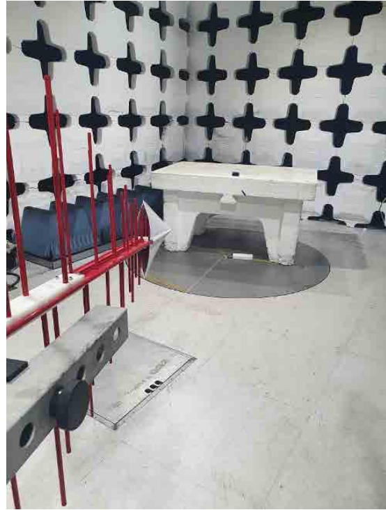
Radiated emissions test set up in 30MHz-1GHz frequency range
