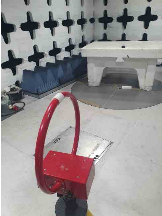
Radiated emissions test set up below 30MHz.
