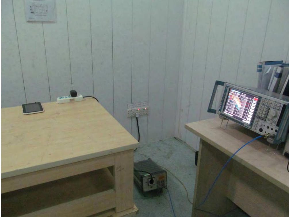
FCC LINE CONDUCTED EMISSION TEST SETUP
