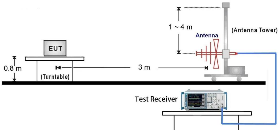
1GHz ~ 18GHz Test Setup:
