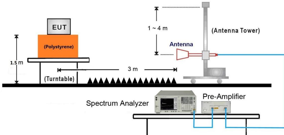
18GHz ~ 40GHz Test Setup:
