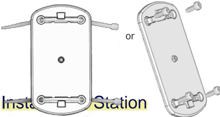
the back groove of base station is aligned with the base card mortise and fixed with the rotation of the clock. connect the USB Power cord and the system will start itself after the power supply.
