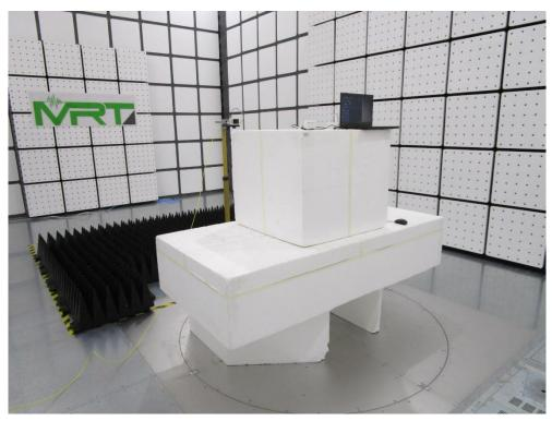
Description: Radiated Emission Test Setup for 18~40GHz
