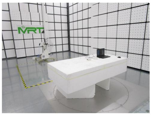
Description: Radiated Emission Test Setup for below1GHz
