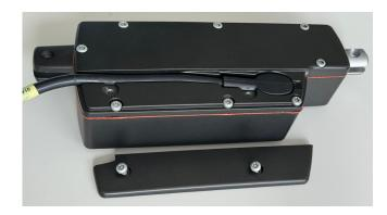
Remove the cable relief by pulling it in the same direction as the screw.
