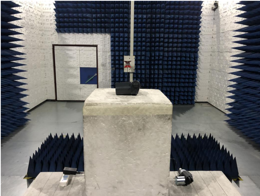
RADIATED EMISSION TEST SETUP ABOVE 1GHZ
