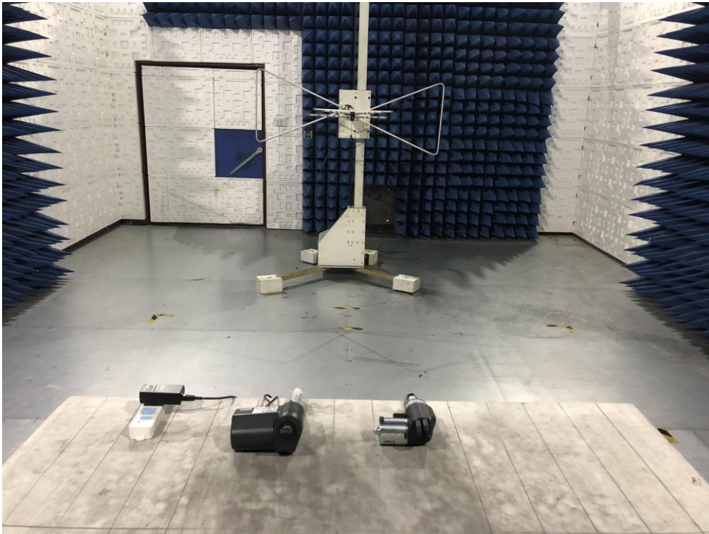
RADIATED EMISSION TEST SETUP ABOVE 1GHZ
