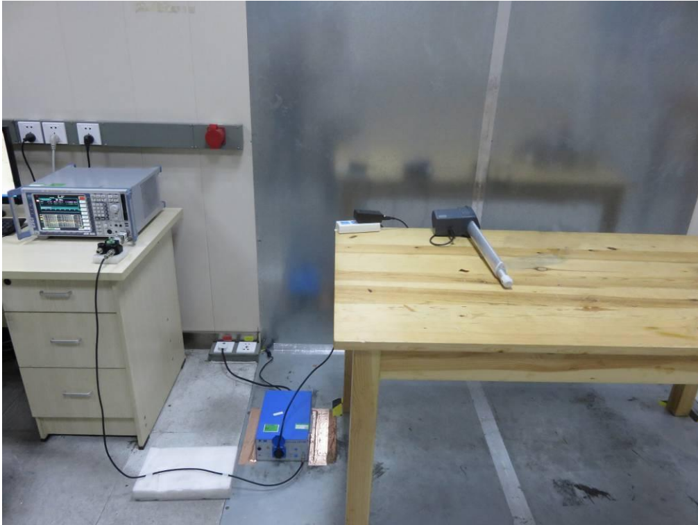
FCC RADIATED EMISSION TEST SETUP
