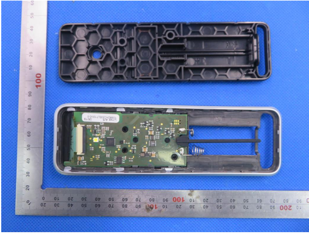
Fig.9 -main board view (type: HC42BL11S000100)
