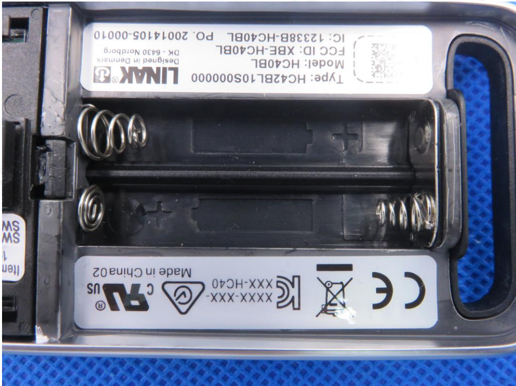
Fig.40 -battery compartment view (type: HC42BL10S000000)
