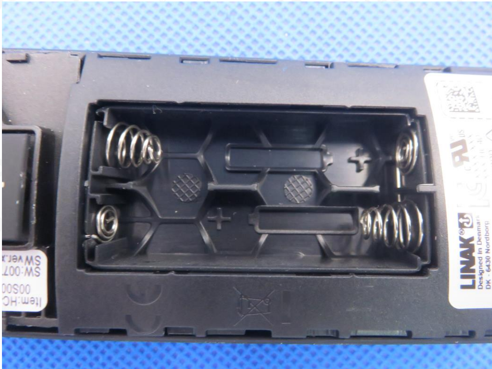
Fig.18 -battery compartment view (type: HC42BL00S000000)
