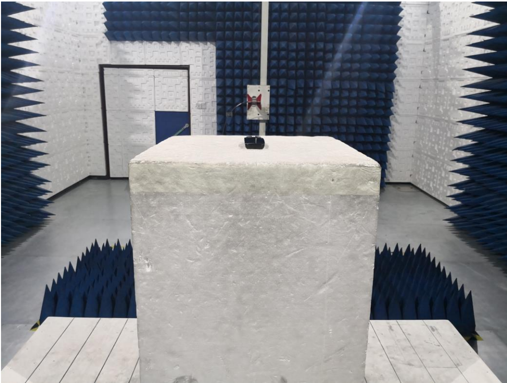
FCC RADIATED EMISSION TEST SETUP ABOVE 1GHZ
