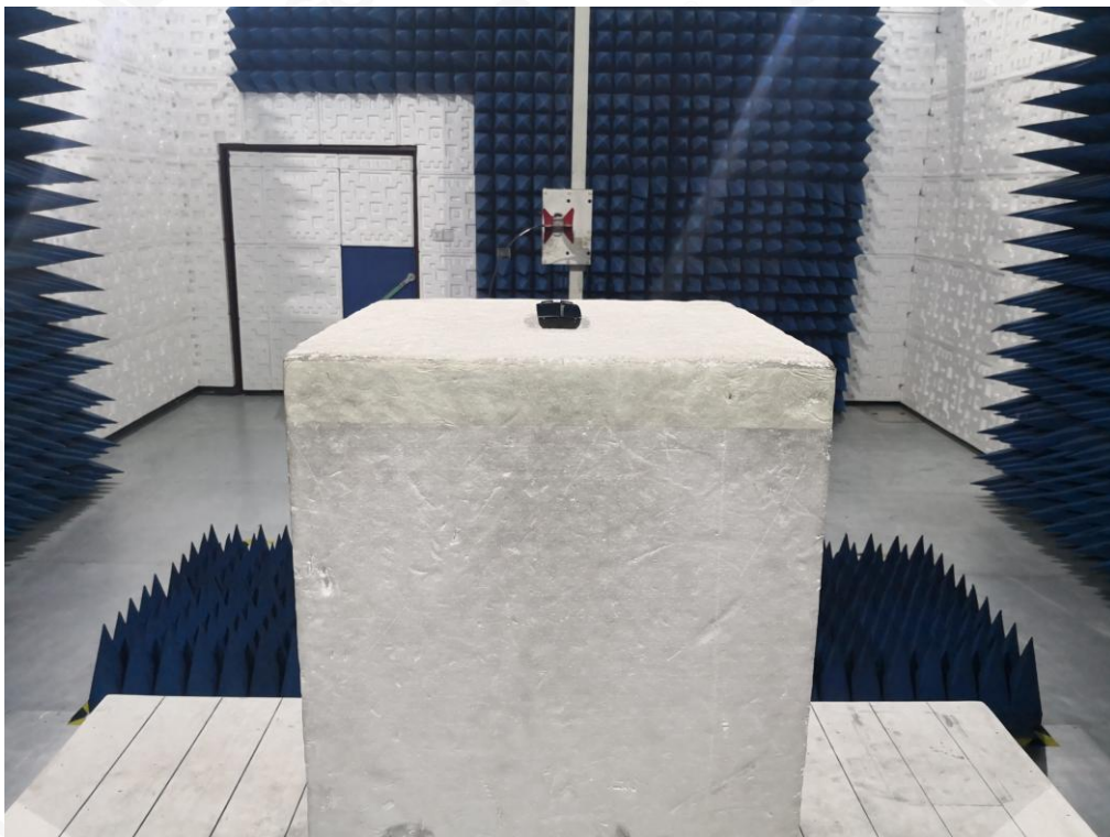
FCC RADIATED EMISSION TEST SETUP ABOVE 1GHZ
