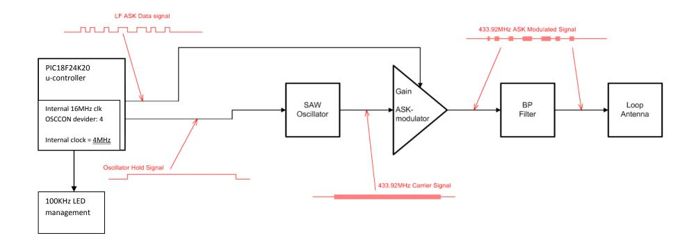
The calibrated internal RC Oscillator provides a 16 MHz clock. The PIC18F system clock can be divided by setting the OSCCON. In this application, the OSCCON is set to 4, and the clock frequency of the CPU is 4MHz.
